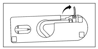
4. Unlock the air compressor hose from the sealant canister by pulling up on the lever.
